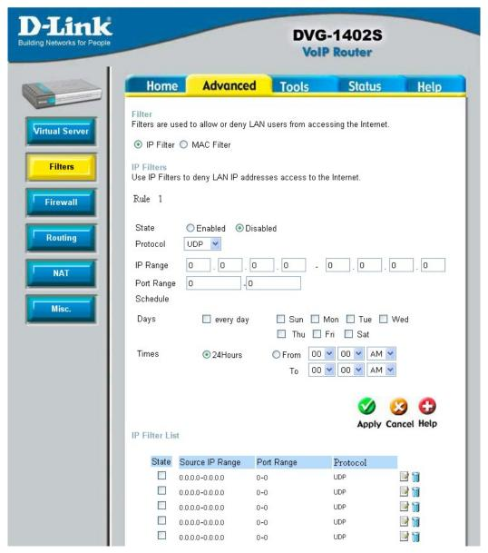
Packet filtering is a basic security measure that should be used on any network that is exposed to a security risk. A packet filter system examines data packets and scrutinizes them in order to control network access. Filtering rules determine whether packets are
